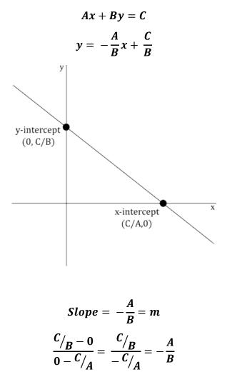
Linear Equation – Straight Line Slope
